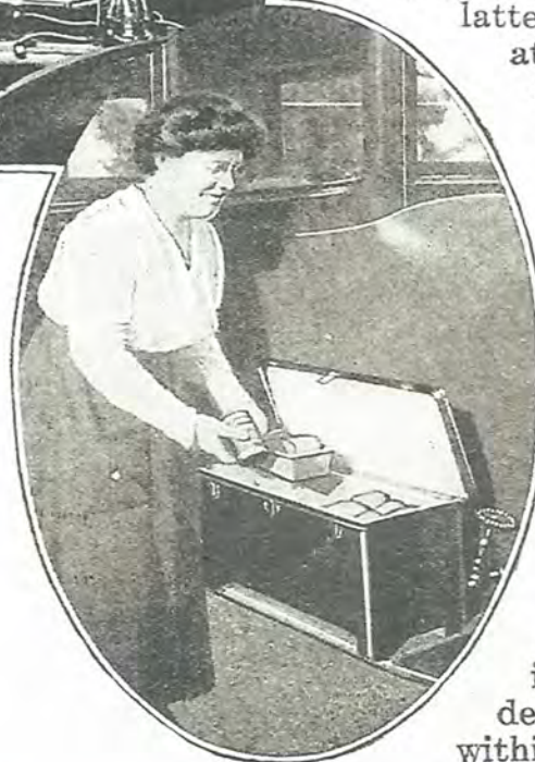
This is the footboard stove. The illustration shows the food being placed in the cooker and the valve that controls the heat
