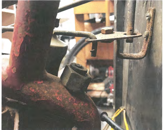
Engine/bike frame and original oiling connection
