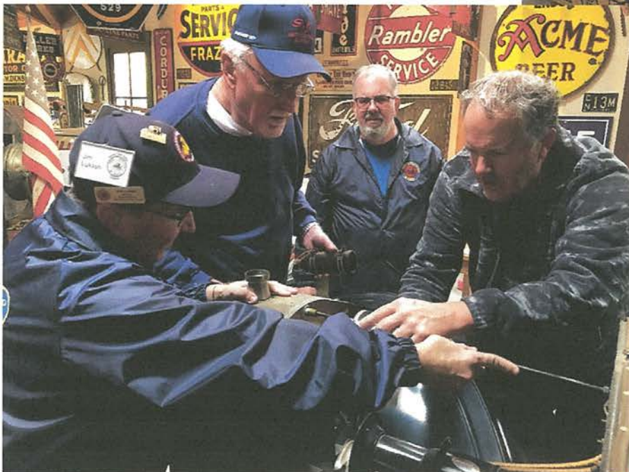
Installing the radiator support rod photo by Ed Harley
