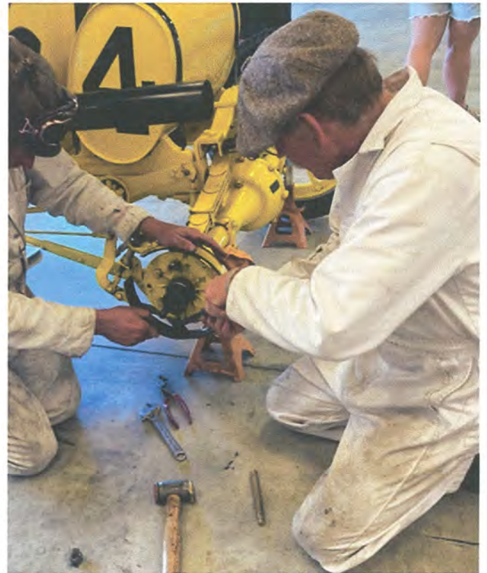
Chris Helling and Bill Bennett removing the brake band for straightening.
