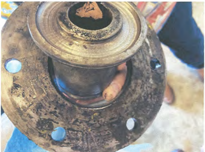
2 piece hub. The flange breaks from the stem. The stem stays on the axle. The flange stays on the wheel.
