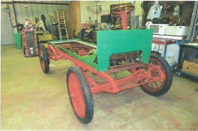
Wheels Mounted on REO
