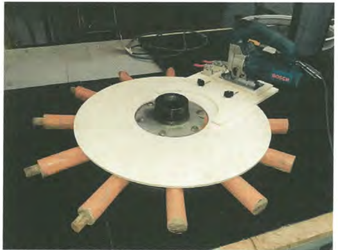
Spoke cutting fixture
