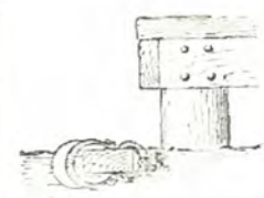
Having done their duty ashore, send 'em to sea. Cut into uniform sizes, laced and hung as illustrated, they make efficient buffers
