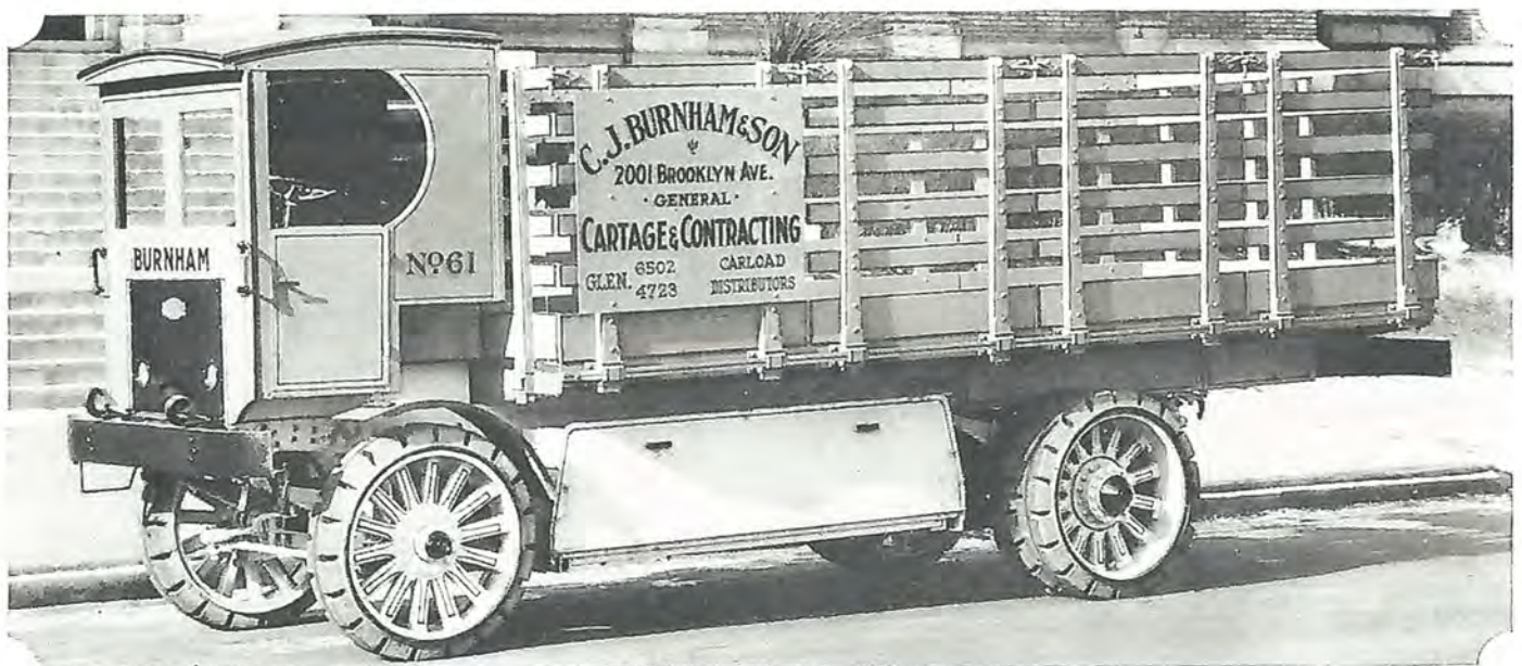
This 10-ton Autocar truck, operated by C. J. Burnham & Son of Detroit, Mich., is said to be the largest electric truck ever delivered west of New York City. The batteries alone weigh 4,065 lbs. Proper tire equipment presented a definite problem which was successfully solved by Kelly Kats.
