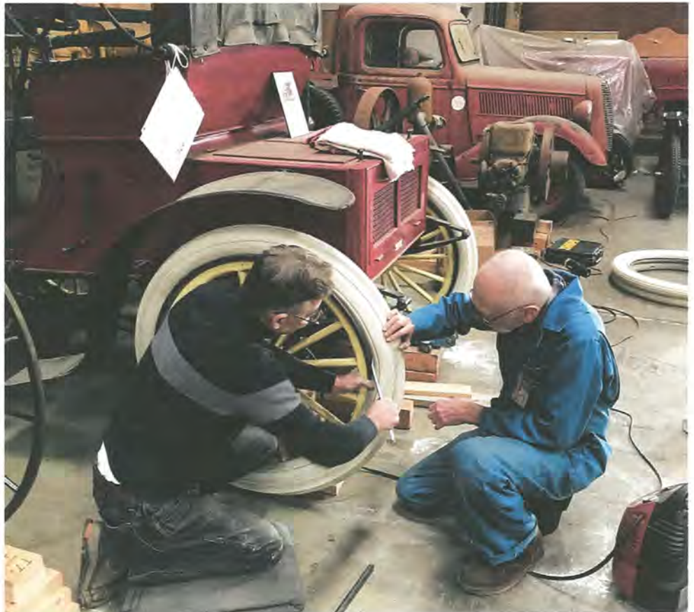
Dan installing a tire with apprentice Allan looking on.
