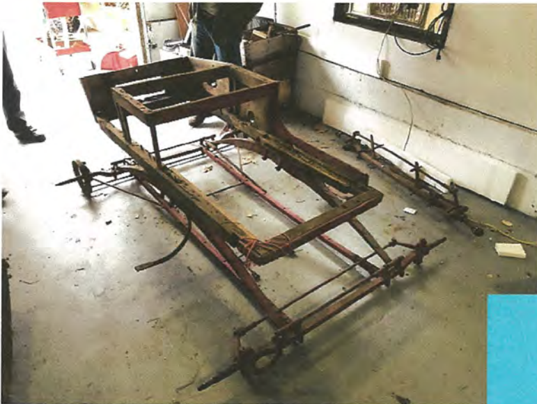
The Frame, as found, with the remains of the Body atop
