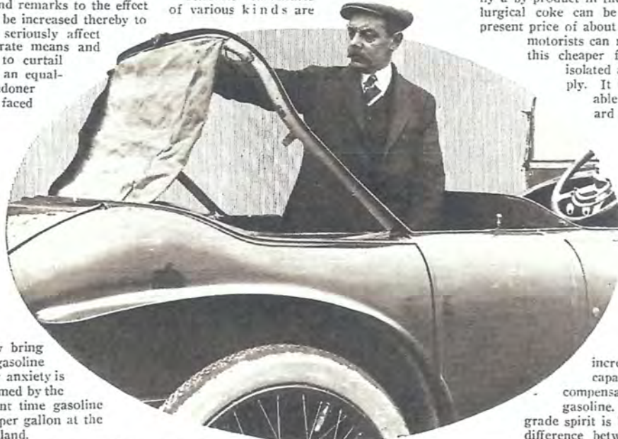
The Turcat-Mery top sinks into a recess and is invisible when down.
