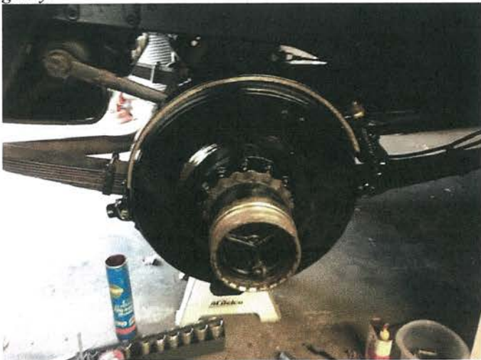
The hubs on Buffalo Wire wheels are fragile. Don't beat on them.
