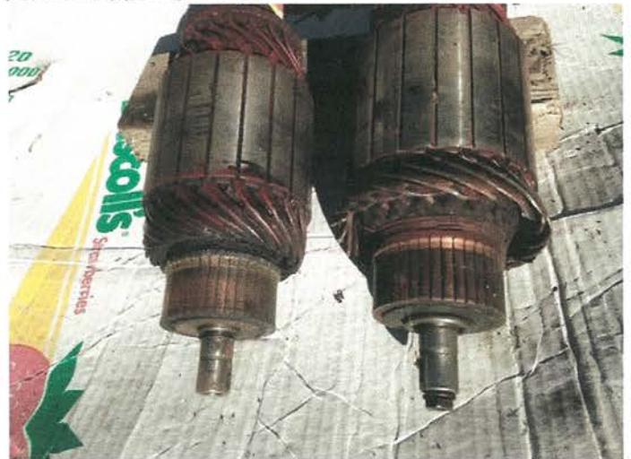
This is what happens to your starter/generator winding if you fail to lubricate the starter gears. The windings have been thrown off of the armature.
