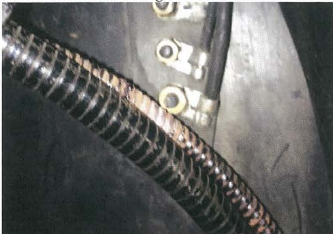
The author's 1926 Willoughby Berline Landaulette was set on fire when the speedometer cable shorted to the lower terminal on the wiring block. The cable clamp shown in the 2nd photo was missing.
