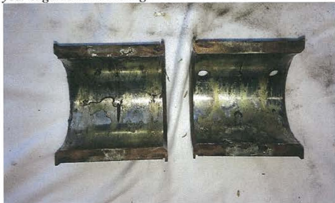
This is what will happen to your center main if you run your car without cleaning out the oil pan and galleys. The bearings got hot enough to melt the babbitt.
