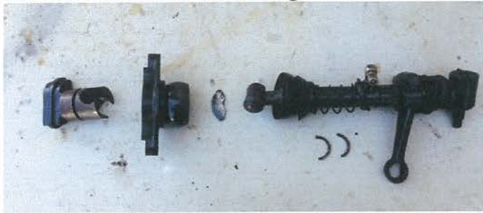
The Perot Links for the front brakes are another part that never gets greased. Replacements are VERY difficult to find.
