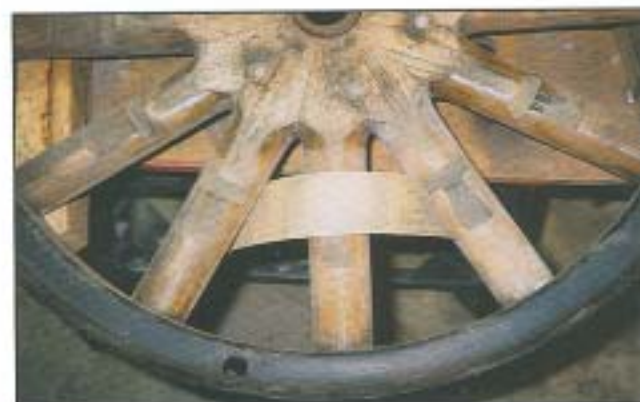
1 1/2" strips of sandpaper for sanding spokes.
